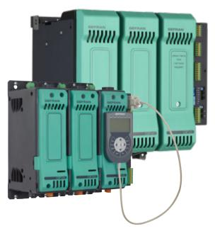
The built-in PID controller option directly acquires the thermocouple or thermoresistance signal and controls power through double SCR junctions while it provides physical relay/logic outputs for alarms and/or cooling functions.
